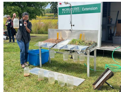
Christine Charles demonstrated water retention of different land-use soils using a Rainfall Simulator. On the left was soil from BAU (business-as-usual) plots, on the right was soil from ASP (aspirational) plots. Photo Credit, YJ Su.
